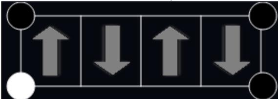
For example, this image shows a configuration, where you will walk the scan path by beginning in the lower left corner (and walking from front to back) in a zig-zag pattern.
